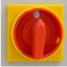
Fig.19. Switch on the control box "0" position
