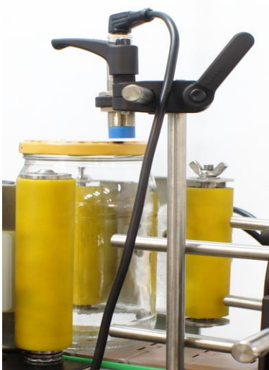
Photo no 4. Setting up the induction sensor
