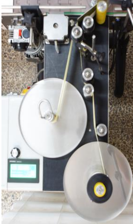
Fig.1. The scheme to place the band with labels
