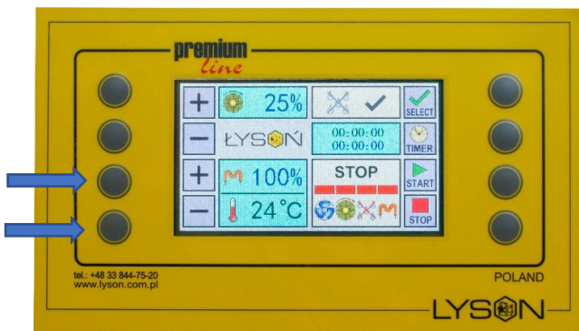
Photo.3 Setting up the heating power and the information on the current temperature inside the device
