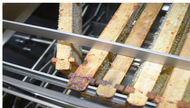
Fig.5 Erroneous frame arrangement in the basket
