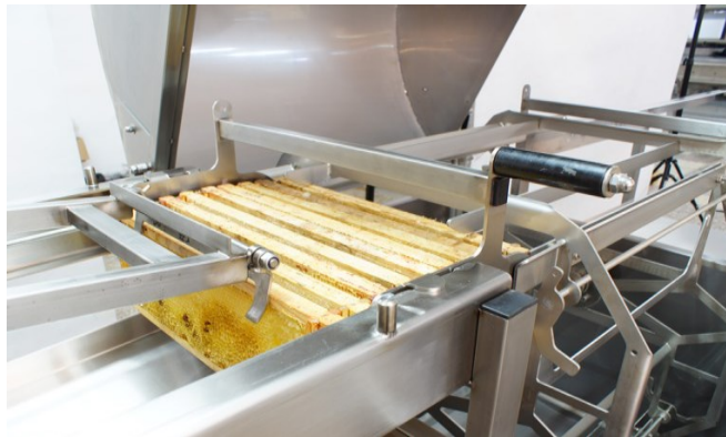
Fig.3 Placing the basket in the position to be blocked
