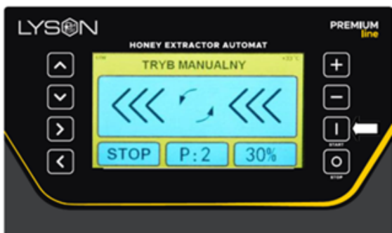
Fig.7 „PLUS” or „MINUS” increasing or decreasing the basket rotations.
