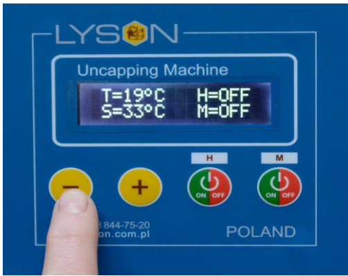
Fig.5. Decreasing the heater temperature Having set the knife heater temperature, switch on the knife heating by button number 3 „ON/OFF”- H . Fig 6. Pressing number 3 button “ON/OFF”- H again will deactivate knife heating (Fig. 6)
