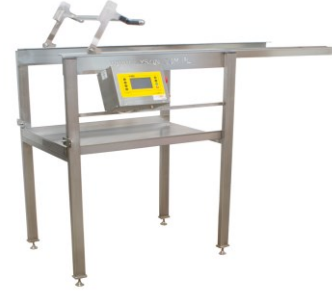
Fig.4. Frame receiver with HE-3 controller
