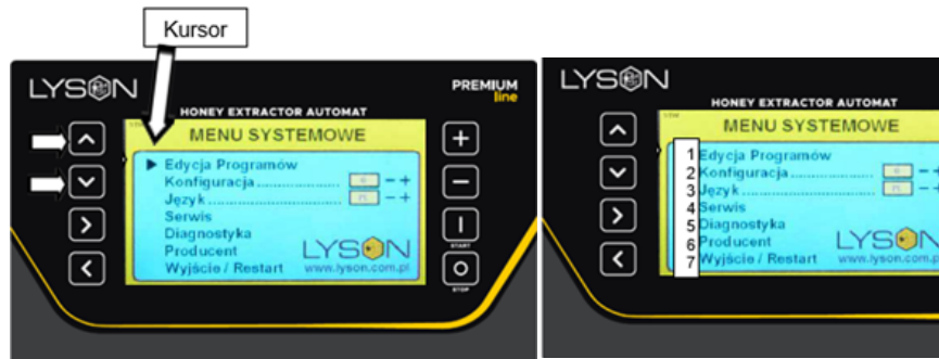
Fig. 13 By means of the buttons „ARROW UP/ARROW DOWN", select the relevant item in the menu Confirm by „START" button – enter the relevant function.
