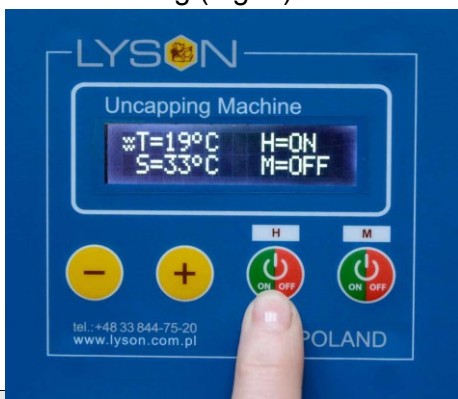
Fig.5. Decreasing the heater temperature Having set the knife heater temperature, switch on the knife heating by button number 3 „ON/OFF”- H . Fig 6. Pressing number 3 button “ON/OFF”- H again will deactivate knife heating (Fig. 6)
