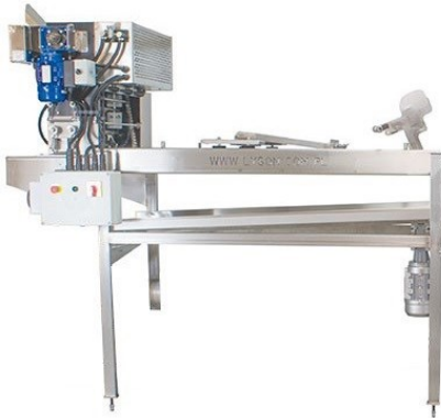
Fig.2. Frame feeder with a loading arm
