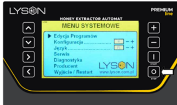
Fig. 13 By means of the buttons „ARROW UP/ARROW DOWN", select the relevant item in the menu Confirm by „START" button – enter the relevant function.
