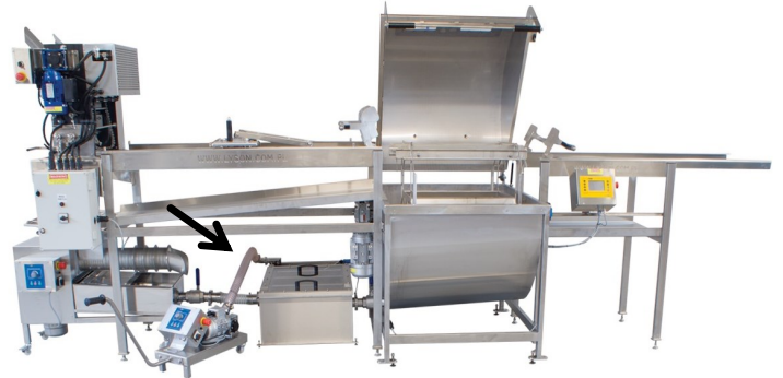
Fig.11. The 'OPTIMA – FULL' line with uncapping machine, insulated strainer, extruder and honey pump, connecting hose marked
