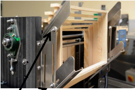
Fig.12. Regulating the upper and lower glide and proper placing of the frames in the glides
