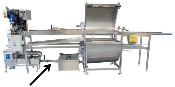
Fig.10. The extractor line with uncapping machine, strainer and extruder, connecting hose marked
