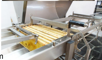
Fig.5 Erroneous frame arrangement in the basket
