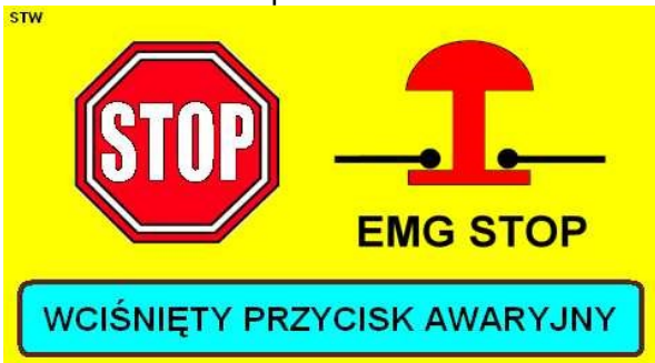
Fig.11 Emergency stop switch pressed – the message displayed after the emergency stop button has been stopped. .
