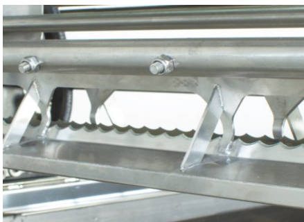
Fig.14. Uncapping machine knives
