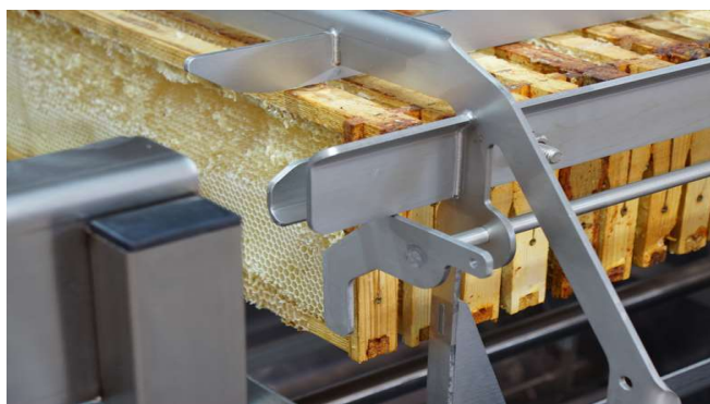
Fig.3 Locking position of the basket
