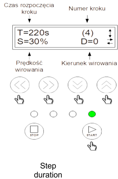
Fig 5. Programming the process cycle sequence – example step (4).
