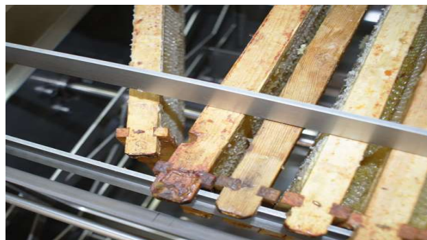
Fig.5 Incorrectly positioned frames in the basket
