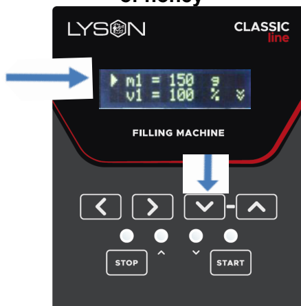
Fig 2. Process flow of dosing the set amount of honey
