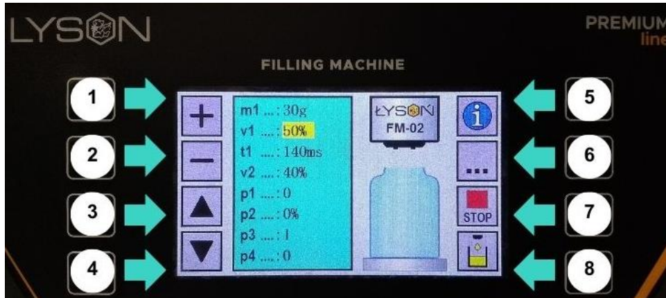
Fot. 5 Button for boost or continuous pump operation (button 8 - press and hold to run the pump continuously)
