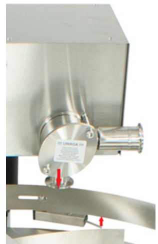
Correctly set limit switch should be located under the dispenser nozzle
