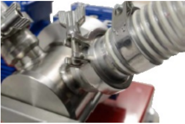
Correct fastening of the hose to the rotor
