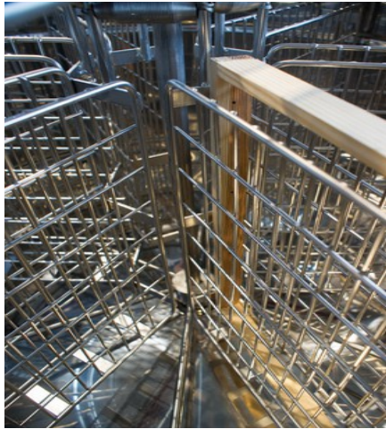
Photo 1. Proper arrangement of frames inside the cassette honey extractor
