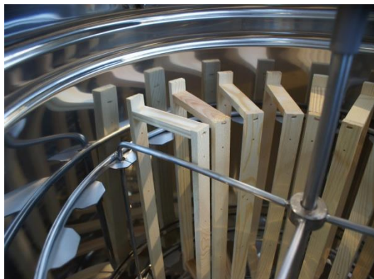
phot.1 Proper frame arrangement inside the radial honey extractor
