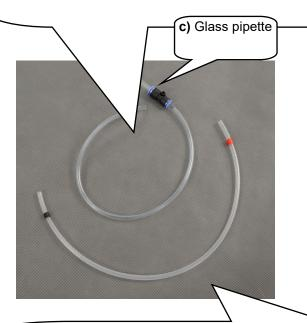
b) hard hose with red and black marking connecting the pump with the bottle
