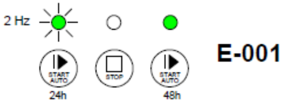
Fig 3. Error - The button to start the creaming cycle 24 h is pressed or blocked
