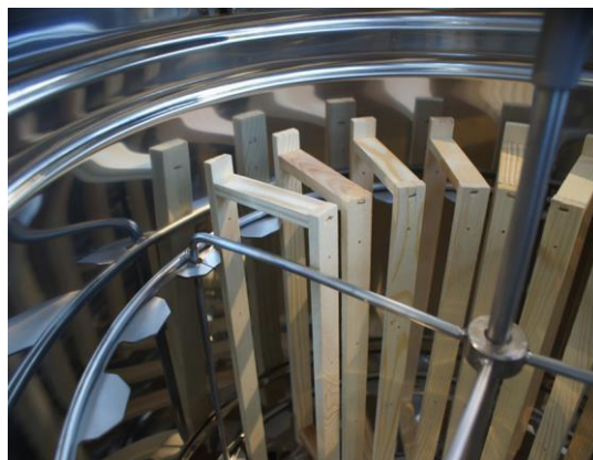
Fig. 2. Proper frame arrangement inside the radial basket
