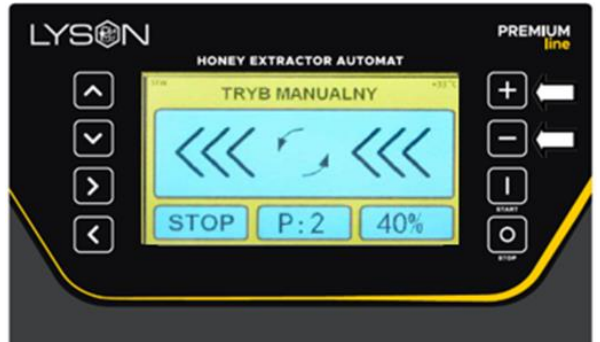
Photo 3 „ PLUS ” or „ MINUS ” increasing or decreasing the basket rotations.
