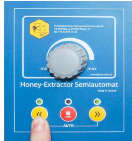
Photo 4. Cassette mode (left and right rotations)
