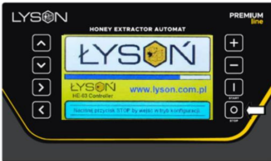
Photo 5 Entering the programming menu
