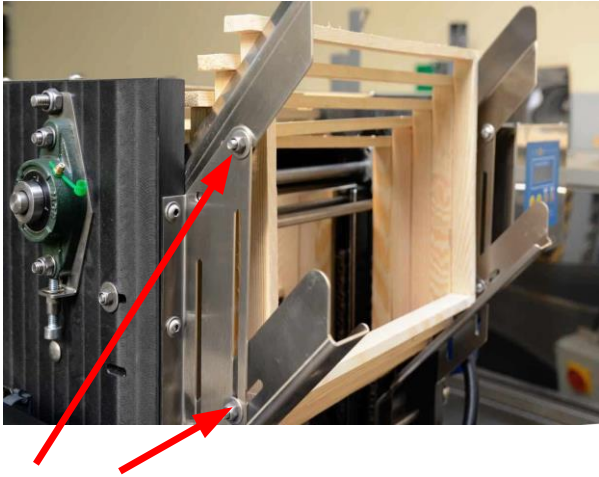
Fig. 13 Adjustment of the upper and lower slide and correct positioning of the frames in the slides
