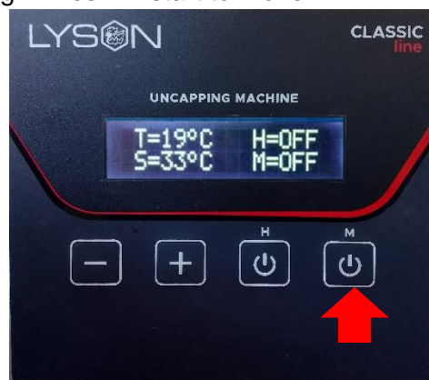
Fig. 10 Switch off the uncapping knives using button no. 4 "ON/OFF".
