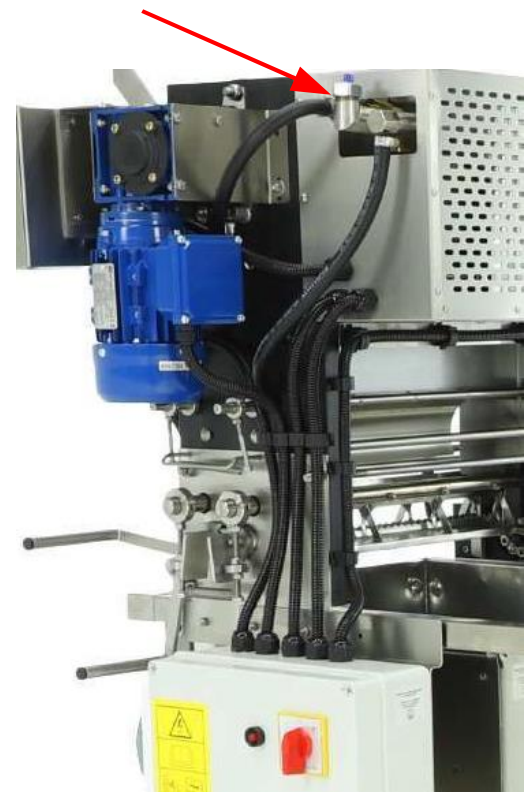
Fig. 21 Fill up port location
