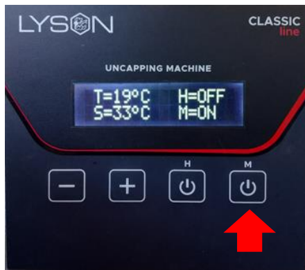
Fig. 9 Switch on the uncapping knives using button no. 4 "ON/OFF".
