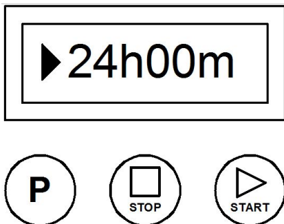
Fig. 2. Depending on the previous set-ups, the screen will display previously preset creaming machine operating time.
