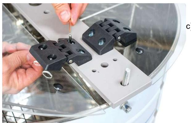
c) tighten the unscrewed hinges again one hole further
