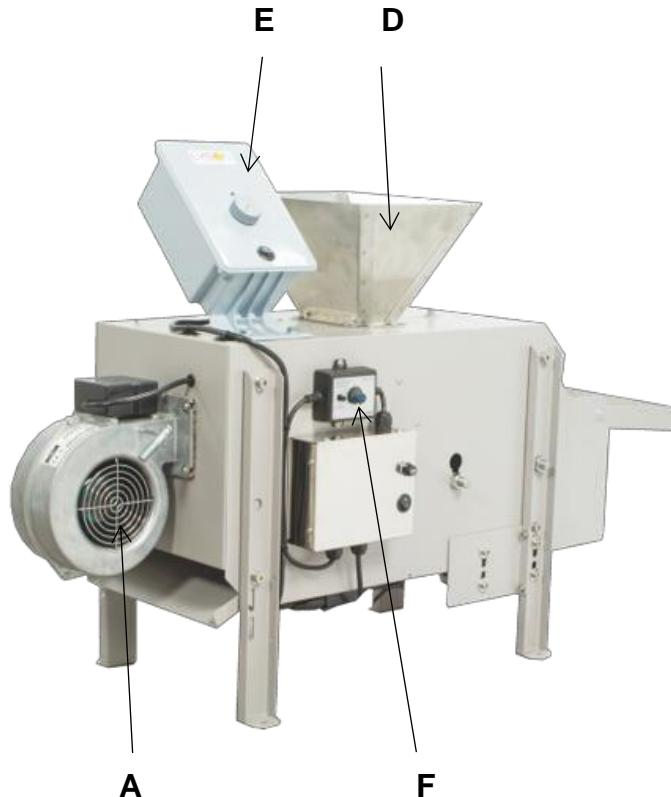
Prior to the first use, clean and dry the device thoroughly. The device shall be washed with hot water with added agents permissible to be used in food industry. While cleaning the device, remember to protect electric elements. After washing, rinse with pure water thoroughly and dry. The device is to be stored in a dry room. None of the device components can be maintained with chemical agents.
