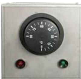
Single-phase thermostats, universal ones. They possess an SPDT (single pole double throw) changeover contact, owing to which they can operate in a heating and cooling modes. Temperature setting by means of a scaled knob. Knob + frame to build in – as a set. Available with different regulation ranges.
