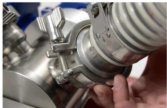
We connect the hose to the rotor with the help of the quick release coupling
