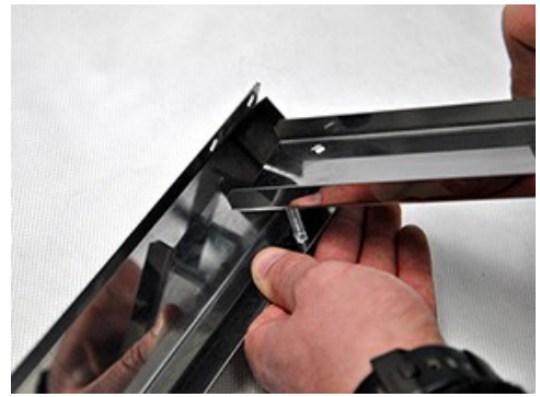
Pic.3. Affix joining components onto the bolts.
