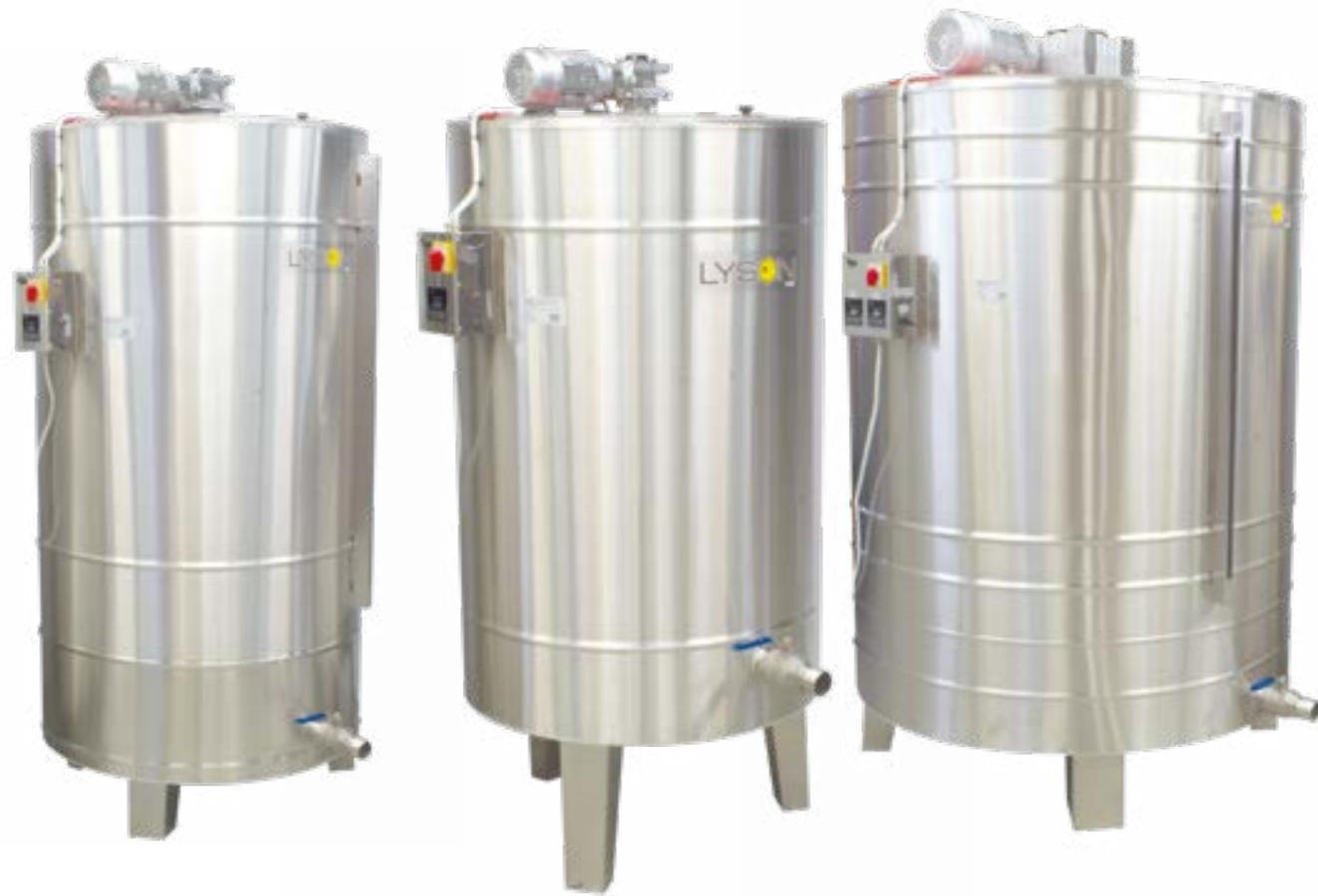
The tanks are made of acid resistant stainless steel. Characteristic feature of the tanks is the conical shaped bottom which allows for effective and hassle free emptying. Tanks are equipped with integrated stainless steel stands, and a matching covers. Tanks are available in four equipment variants. Brushed steel outer surface. Tanks 1000 are equipped with level indicator.
