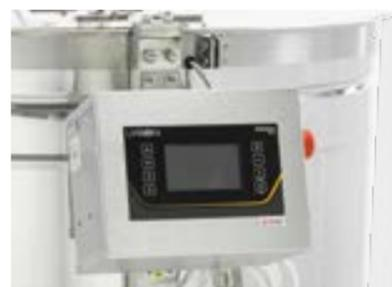
HE-03 controller has 7 fully modifiable automatic programs and 2 manual programs. Large (4,3") colour display, simple and intuitive interface significantly enhances the comfort of using it. Additionally the controller has the functionality of work time counter for both motor and controller. Advanced diagnostic and monitoring tools control the work parameters of motor and controller. The controller is equipped with top quality Mitsubishi inverter.
