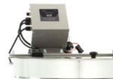
Controller dedicated for OPTIMA Line extractors. Dual power 12V / 230V. Two manual Left and Right modes. No factory pre-set programs. To set up the programs press "+" and "-" buttons simultaneously on the controller's start up.
