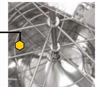
Basket made of rod 10mm acid-resistant stainless steel in which 24 Dadant US frames can be inserted and 42 frames of type Langstroth, Deutsch Normal, ZANDER, D 1/2. The basket is supported by a 2 bearings.
