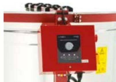
The honey extractor can be operated both in manual mode (2 programs) and in automatic (1 program). In manual mode, you can set the direction and speed (using the knob). The predefined auto program is set by manufacture. The automatic mode is activated by simultaneously pressing both directional buttons. The controller works with a high class Mitsubishi inverter.
