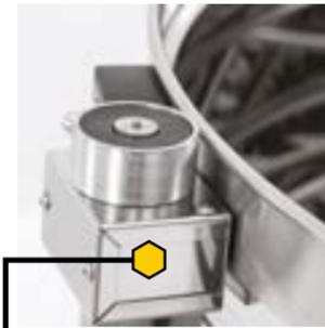
Electromagnetic interlock - prevents opening of the extractor during operation
