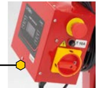
A modern controller, which allows you to change the direction of the basket, so that the cassette swings to the right side once to the left side, there is no need to manually rotate the frames! The controller has 10 automatic programmes and two manual programmes (right-left)
