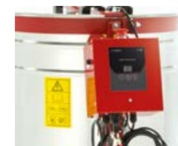
Dual power controller 12V/230V dedicated for tangential and radial honey extractors of 500 to 900 mm extractors. Digital 10 step speed adjustment.
