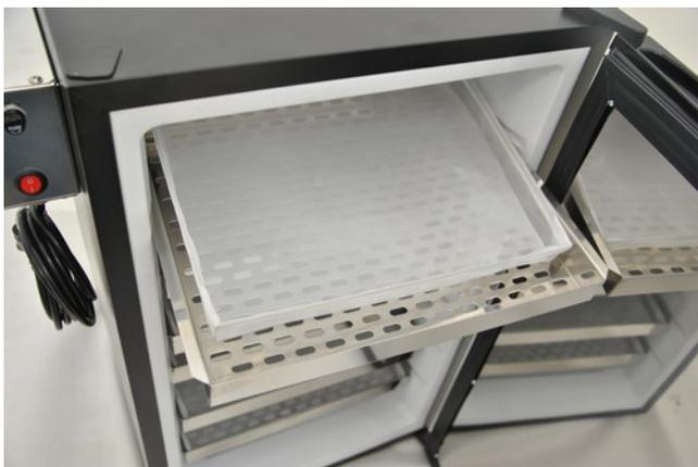
Dryer holds inside 6 drawers made of stainless steel, acid resistant :
