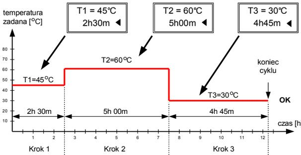
Fig.1 An example of the heating cycle: T1 = 45 ° C, 2h30m -> T2 = 60 ° C, 5h00m -> T3 = 30 ° C, 4h45m.
