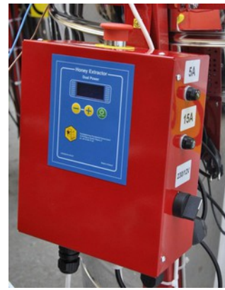
fot. 5 5A, 15A fuses (side pannel)
