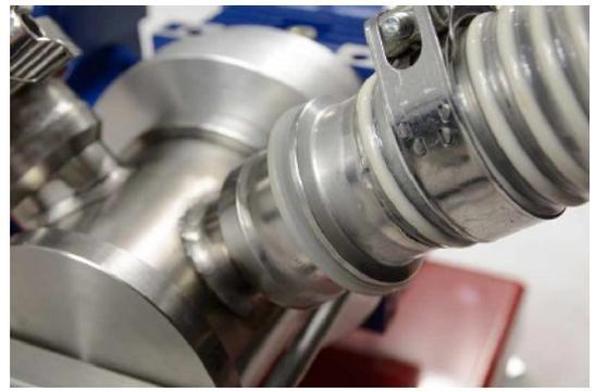
Place the hose end on the pumping unit nozzle
