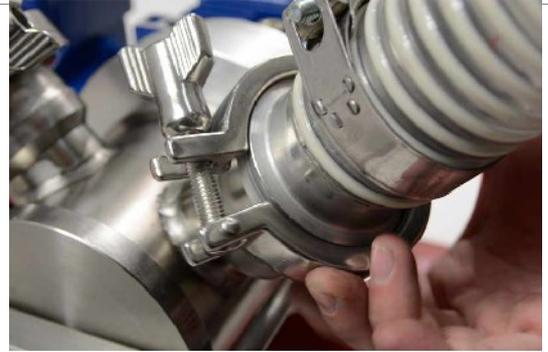
Secure the hose using the quick connector (supplied)
