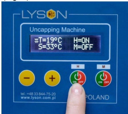
Fig. 7 H=ON message as well as a graphical icon will be displayed after turning knife heaters ON.
