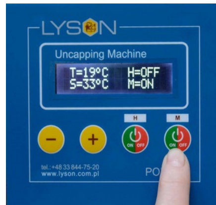
Fig. 9 Press „ON/OFF” button (#4) to turn uncapping knives on. M=ON is displayed when uncapping knives are working. Be aware that the knives are now in motion.
