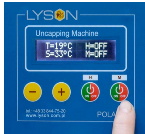
Fig. 10 To turn uncapping knives off press „ON/OFF” button (#4) again. M=OFF message is displayed when knives are stopped.
