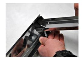
**Pic.3.** Affix joining components onto the bolts.
