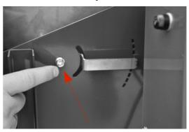
Loosen the screw located just behind the inclination adjustment to change the level the sieve is fixed at as per photo above. Having done so, do not forget to tighten the bolt!
