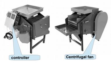
Electrically powered fan generates a blow which throws the contaminated debris out of the sieves. Pollen falls down onto an inclined plane located in the bottom part of the cleaner.
