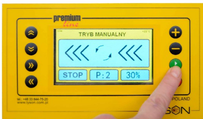
Fot.2 Switching on the extractor.
