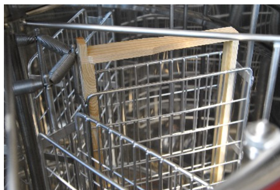
Fig. 2 Correct frames arrangement in the cassette basket
