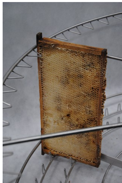
Fig. 1 Correct frame arrangement in the radial basket
