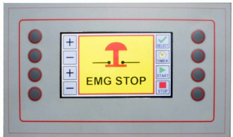
Fot.9 Emergency Button active – warning message
