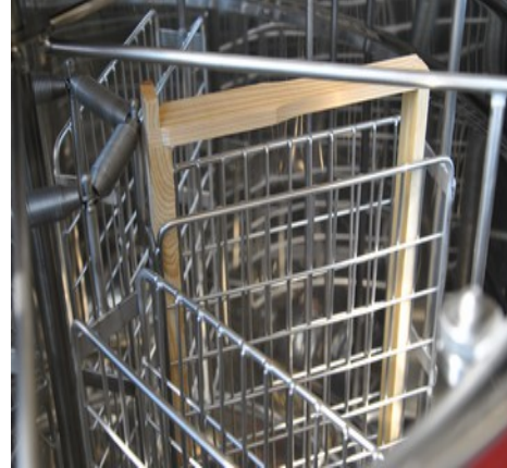
Fig.1. Correct frame arrangement in Cassette Extractor
