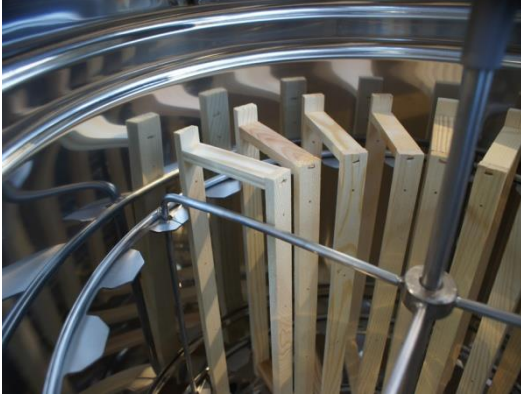
phot.1 Proper frame arrangement inside the radial honey extractor
